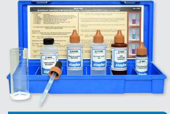
Use the K-1582 to ensure quaternary ammonium-based equipment/facility sanitizers do not exceed 200 ppm if you want to avoid a water rinse.
