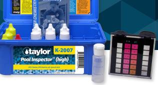
K-2007: Tests are performed in the #9056 comparator block. Kit may be used to test both chlorine and bromine.
